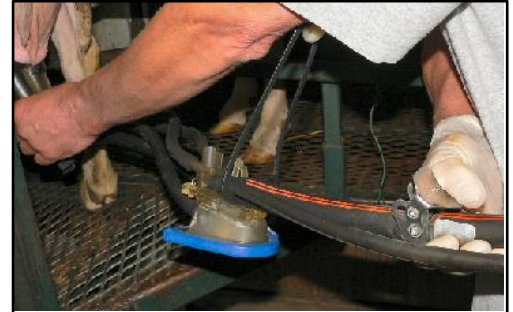
Fig. 1. Using shut-off valve to remove unit
