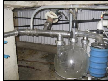
Fig. 15. Keep air injectors clean
